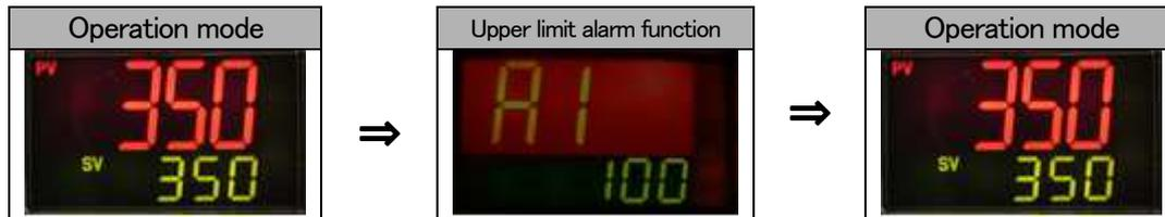
Upper limit alarm: It alarms when the temperature exceed the range of the set temperature.
