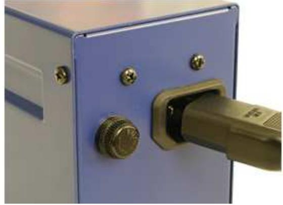
② Connect the soldering iron unit (LS-90) to the 5P connector at front.
