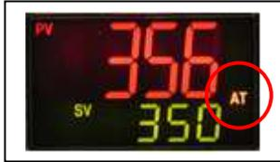
Auto-tuning: It automatically calculates suitable PID value which controls soldering iron.
