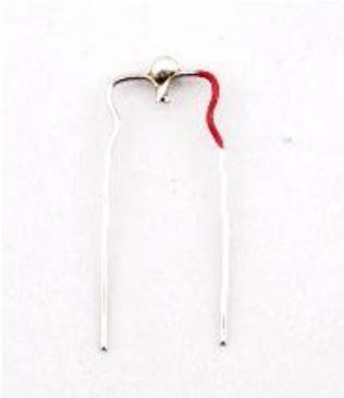
Impurities of solder dust and flux will be stained to iron tip sensor (SC-006). Keep SC-006 clean in order to measure the temperature accurately.
