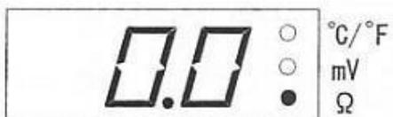
※ In case that the tester generates its own resistance at ②,③, nullify the resistance by simultaneously holding down the earth line resistance measurement button (red) and the ZERO adjustment button (black) for approximately 2 seconds.
