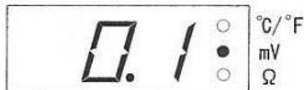
Connecting earth clip and LR pin, and press leak voltage measurement button (yellow), display indicates 0~0.1mV.
