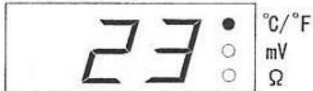
Setting power switch on, then display indicates near-room temperature.
