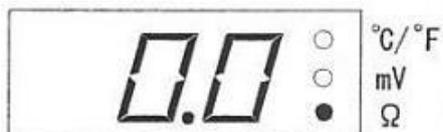
Connecting earth clip and LR pin, and press Earth line resistance measurement button (red), display indicates 0Ω.
