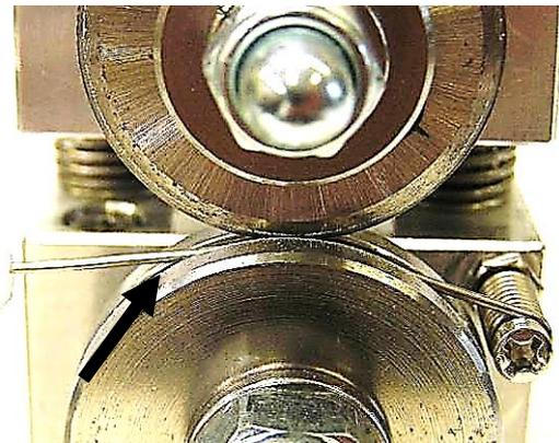
Feed the solder wire by pressing the foot switch.
