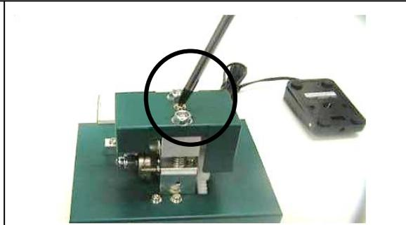
2) In order to remove the V-blade from the upper housing, loosen the adjuster screws alternately until having enough space between the V-blade and the guide pulley.
