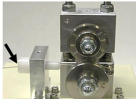
2) Lead the solder wire along the groove of the guide pulley and V-blade little by little by pressing the foot switch.
