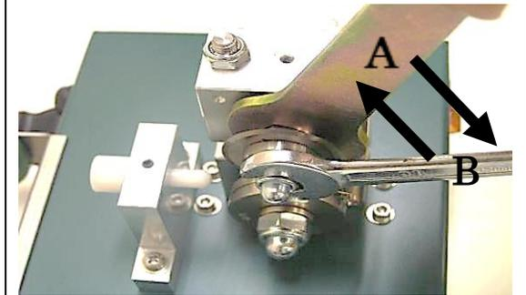
4) Fix the new V-blade firmly while pushing each wrench in the direction of the arrows.
