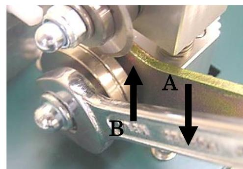
5) Fix the new guide pulley firmly while pushing each wrench in the direction of the arrows.
