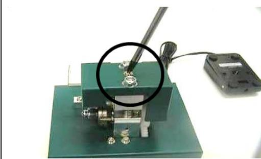
2) In order to remove the guide pulley from the lower housing, loosen the adjuster screws alternately until having enough space between the V-blade and the guide pulley.
