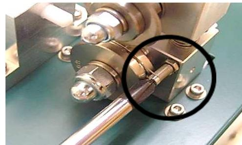
4) Hold the guide pulley shaft with a wrench A and the guide pulley holder with a wrench B.
