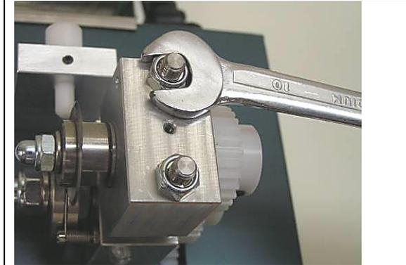
3) Hold the V-blade shaft with a wrench A and the V-blade holder with a wrench B. Remove a cover nut of the V-blade holder while pushing each wrench in the direction of the arrows. Remove the V-blade and exchange with a new one.
